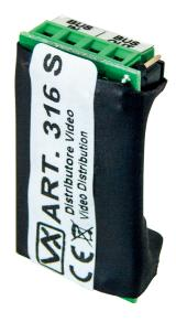
1 Way video distributor for systems with balanced video signal (4+1 or VX2200). It allows to connect one videophone on a balanced video network keeping the same line impedance.
